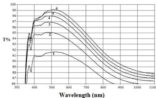
**Figure 1.** Light transmission of uncoated glass (curve 1) and coated glasses (curves 2–6) obtained from silica sols with ALM-10 additives (wt.%): 2 - 1.0; 3 - 1.5; 4 - 2.0; 5 - 2.5; 6 - 3.0
