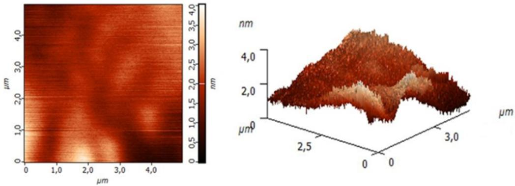
**Figure 6.** AFM image of the surface of the coating obtained from the silica sol with the addition of ALM-2 (3.0 wt.%)
