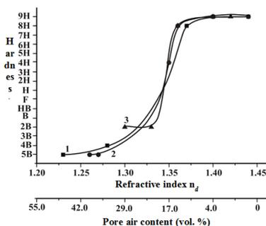
**Figure 4.** Dependence of hardness of antireflection coatings obtained from silica sols with additives of ALM-10 (curve 1), ALM-7 (curve 2), ALM-2 (curve 3), on the refractive indices and pore air content
