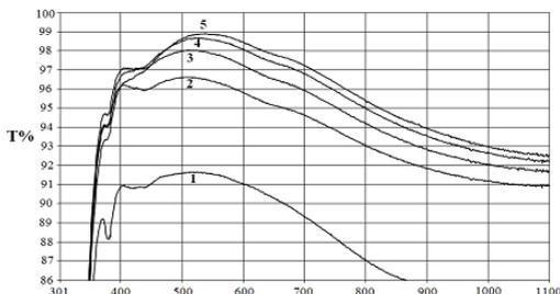
**Figure 3.** Light transmission of uncoated glass (curve 1) and coated glass (curves 2–6) obtained from silica sols with ALM-2 additives (wt.%): 2 - 1.0; 3 - 1.5; 4 - 2.0; 5 - 3.0
