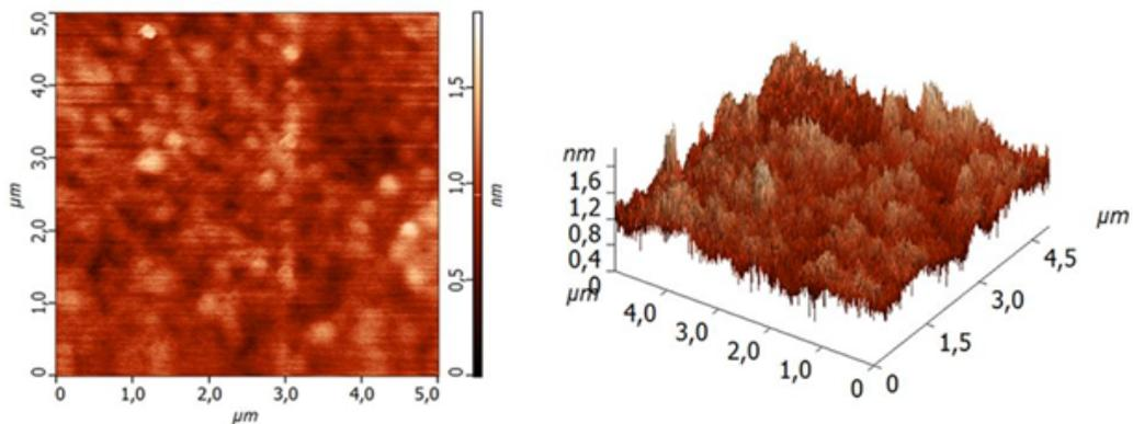
**Figure 5.** AFM image of the surface of the coating obtained from the silica sol with the addition of ALM-2 (1.0 wt.%)
