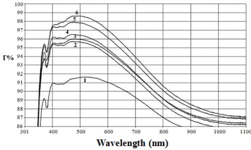
**Figure 2.** Light transmission of uncoated glass (curve 1) and coated glasses (curves 2–6) obtained from silica sols with ALM-7 additives (wt.%): 2 - 1.0; 3 - 1.2; 4 - 1.5; 5 - 2.0; 6 - 3.0
