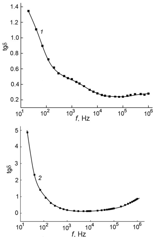
**Fig. 3.** Frequency dependences of dielectric loss angle tangent in  $(1-x)\text{TlGaSe}_2 \cdot x\text{Dy}$ :  $x = 0$  (1) and  $0.03$  (2).  $T = 298$  K.
