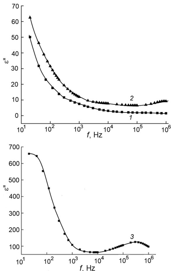
**Fig. 2.** Frequency dependences of the imaginary component of the complex dielectric permittivity of crystals  $(1-x)\text{TlGaSe}_2 \cdot x\text{Dy}$ :  $x = 0$  (1);  $0.01$  (2) and  $0.03$  (3).  $T = 298$  K.
