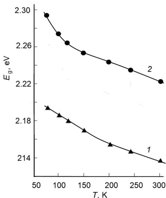
**Fig. 5.** Temperature dependences of the band gap for  $\text{TlGaSe}_2$  (1) and  $0.99\text{TlGaSe}_2 \cdot 0.01\text{Dy}$  (2) crystals.
