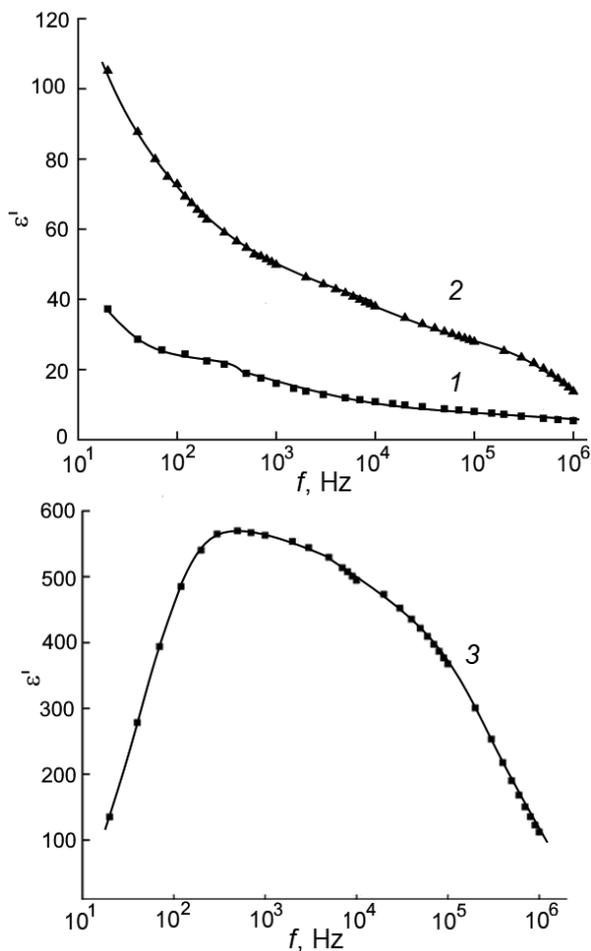
**Fig. 1.** Frequency dependences of the real component of the complex dielectric permittivity of crystals  $(1-x)\text{TlGaSe}_2 \cdot x\text{Dy}$ :  $x = 0$  (1); 0.01 (2) and 0.03 (3).  $T = 298$  K.
