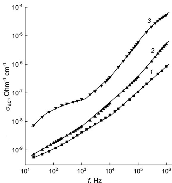
**Fig. 4.** Frequency dependence of the conductivity of crystals  $(1-x)\text{TlGaSe}_2 \cdot x\text{Dy}$ :  $x = 0$  (1);  $0.01$  (2) and  $0.03$  (3).  $T = 298$  K.
