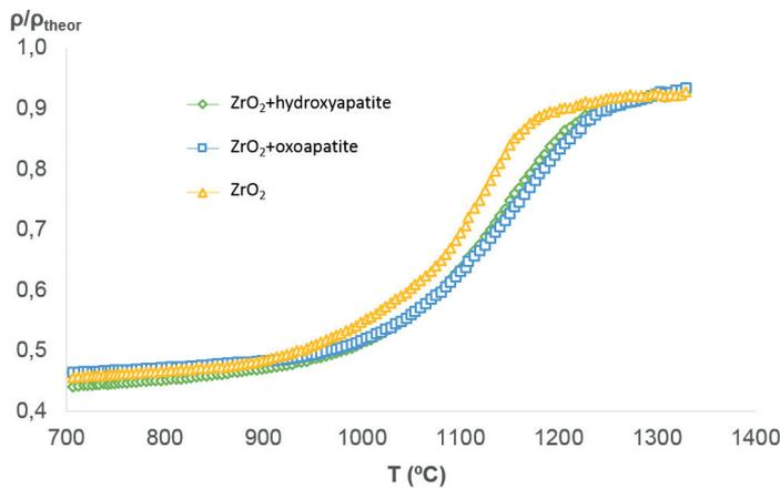
**Figure 3.** Graph of temperature dependence of relative density of samples during sintering of ceramics
