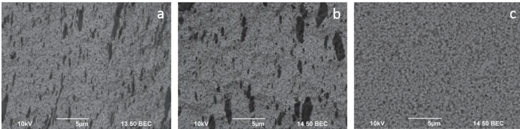
**Figure 5.** Microimagies of surfaces of ZrO<sub>2</sub>/HAp (a), ZrO<sub>2</sub>/OAp (b) and ZrO<sub>2</sub> (c) ceramics
