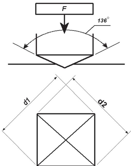
**Figure 1.** Scheme of indenter indentation into the sample.
